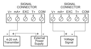
Transmitter Powered by External Supply
