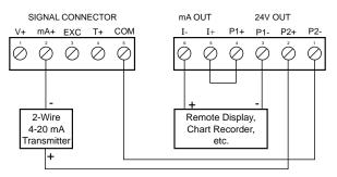
4-20 mA Output & Input Signal Powered by Meter
