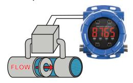
In this application, the PD8-765 is displaying flow rate by extracting the square root from the 4-20 mA signal from a differential pressure transmitter. The user selectable low-flow cutoff feature gives a reading of zero when the flow rate drops below a user selectable value.
