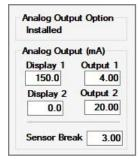
The meter can be set up for reverse scaling as shown to the left: the output will be 4.00 mA when the display reads 150.0 and the output will be 20.00 mA when the display reads 0.0
