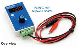
The PD9502 is a low-cost, compact, simple to use 4-20 mA or 0-10 VDC signal generator. It can easily be set for 0-20 mA, 4-20 mA, 0-10 V or 2-10 V ranges. Signal adjustment is made with a one-turn knob. A 15-27 VDC wall plug is provided with the instrument. Optional USB power bank is available.
