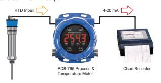
The 4-20 mA output can be reversed scaled such that 4 mA represents the high value and 20 mA represents the low value. For instance, a 4-20 mA output signal could be generated as the meter went from 100.0 to 0.0.
