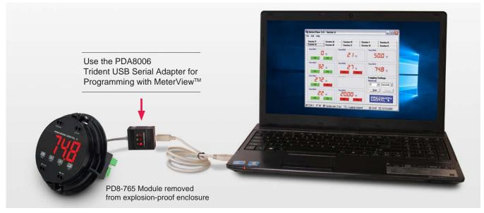
Note: PD8-765 meter is not powered from USB connection and requires external power to be programmed.
