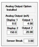
When a meter is programmed as shown to the left, the output will be 4.00 mA when the display reads 0.0 and the output will be 20.00 mA when the display reads 150.0.
