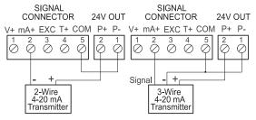
Transmitter Powered by Internal Supply (optional)
