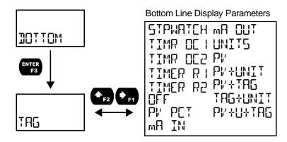
The bottom line (IIIII) can be programmed to display:
