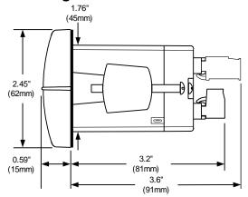
Figure 2. Meter Dimensions - Side View
