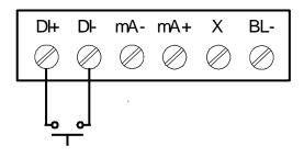
**Figure 7. Digital Input Connections**
