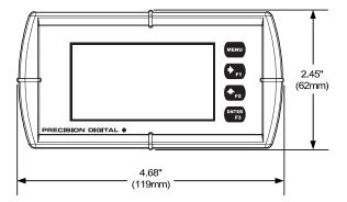
Figure 3. Meter Dimensions - Front View
