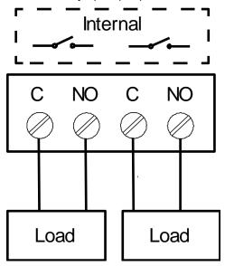
Figure 9. Solid State Relay Connections
