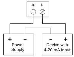
Figure 8. 4-20 mA Output Connections
