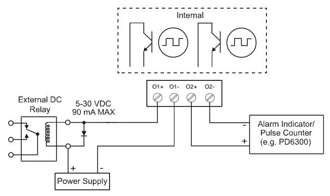
Figure 10. Open Collector Output Connections
