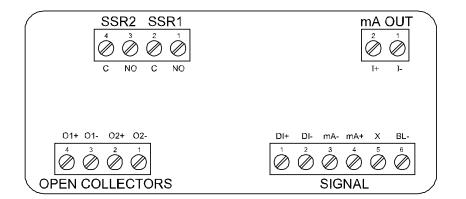
Figure 4. Connector Labeling for Fully Loaded Meter
