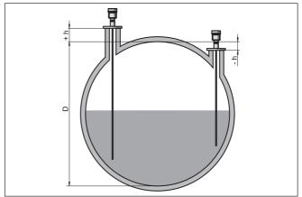
Fig. 16: Vessel height and socket correction value
