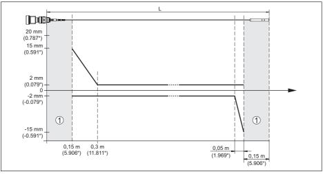
Fig. 27: Deviation NivoGuide 3100 in cable version
