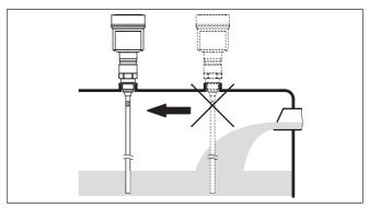
Fig. 7: Mounting of the sensor with inflowing medium
