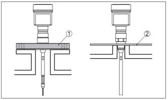
Fig. 3: Mounting in non-metallic vessel
