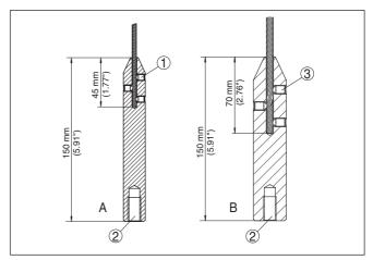
Fig. 20: Shortening the cable probe
