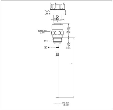
Fig. 34: NivoGuide 3100, rod ø 16 mm (0.63 in), threaded version
