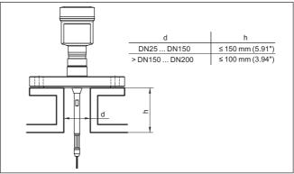
Fig. 5: Mounting socket
