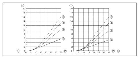
Fig. 22: Max. tensile load with sand and cement - Cable: ø 4 mm (0.157 in)
