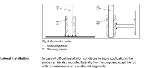
To compensate for the resulting changes in signal runtime, let the instrument determine the probe length automatically.
