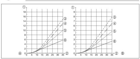
Fig. 23: Max. tensile load with cereals and plastic granules - Cable: ø 6 mm, ø 11 mm, PA coated
