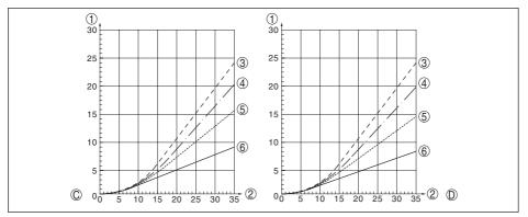
Fig. 24: Max. tensile load with sand and cement - Cable: ø 6 mm, ø 11 mm, PA coated
