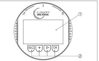
Fig. 15: Display and adjustment elements
