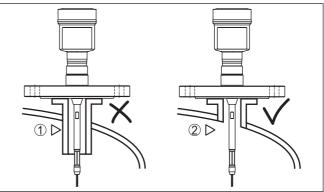
Fig. 6: Socket must be installed flush
