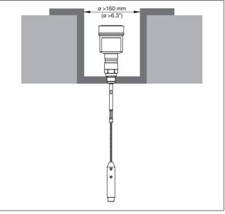
Fig. 4: Mounting in concrete silo
