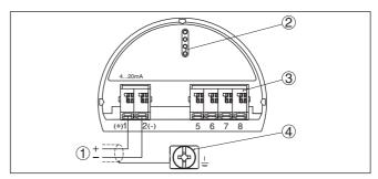
Fig. 10: Electronics and connection compartment - single chamber housing
