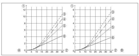
Fig. 21: Max. tensile load with cereals and plastic granules - Cable: ø 4 mm (0.157 in)
