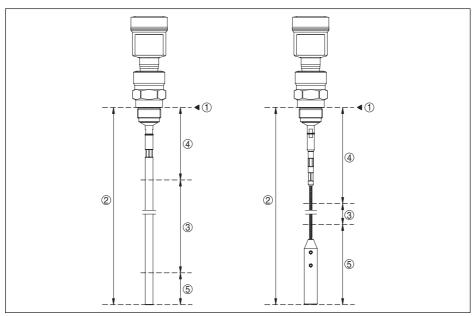
Fig. 25: Measuring ranges - NivoGuide 3100
