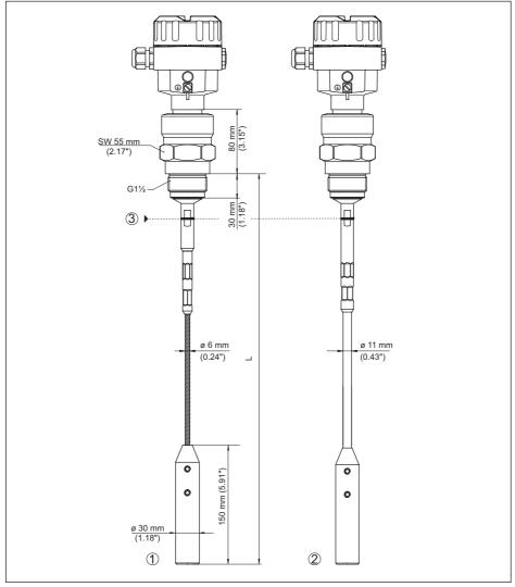
Fig. 33: NivoGuide 3100, cable Ø 6 mm (0.236 in), Ø 11 mm (0.433 in) threaded version with gravity weight (all gravity weights with thread M12 for eye-bolt)
