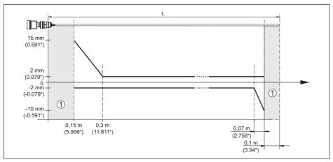
Fig. 26: Deviation NivoGuide 3100 in rod version
