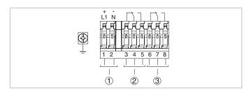
Wiring plan, single chamber housing
