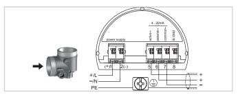
Connection compartment with double chamber housing - mains voltage
