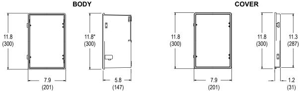
Dimensions for: PDA2301, PDA2301-V, PDA2302, PDA2302-V, PDA2303, PDA2303-B, PDA2322.
