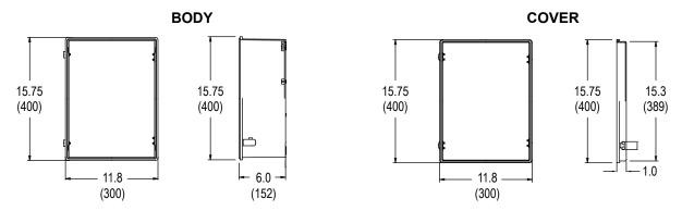
**Dimensions for:** PDA2303-V, PDA2304, PDA2304-V, PDA2304-1, PDA2304-2, PDA2304-3, PDA2305, PDA2305-V PDA2306, PDA2306-V, PDA2307, PDA2308, PDA2308-B, PDA2312.
