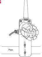
Figure 1. PDA6963 Mounted to 2" Horizontal Pipe
