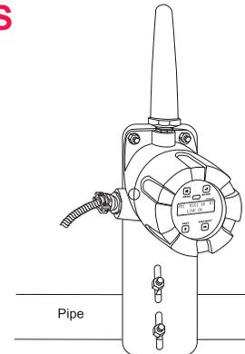
Figure 1. PDA6963 Mounted to 2" Horizontal Pipe
