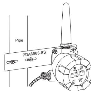
Figure 2. PDA6963 Mounted to 2" Vertical Pipe.
