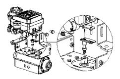
7. Tighten the positioner and the bracket with hexagon-headed bolts and plate washer **after checking the positioner**'s **position**.
