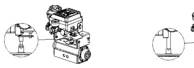
Fig. 5: Fork lever type (left) and NAMUR lever type (right)
