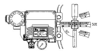
8. Check the valve stroke. The stroke marks are indicated on the feedback lever of the positioner. Position the connection pin at the number on the feedback lever which corresponds to the desired valve stroke. To adjust, move the bracket, the connection pin or both.
