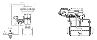
Fig. 7: Singe acting linear (left) and rotary (right) type actuator
