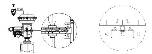
Proper way to connect feedback lever, connection pin, and lever spring
