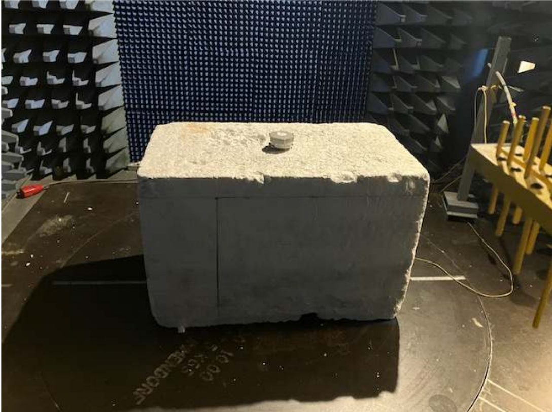
Figure 1: Radiated Immunity Test
