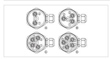
Connection compartment of the probe - 220  $k\Omega$  resistance between terminals 1 and 2
