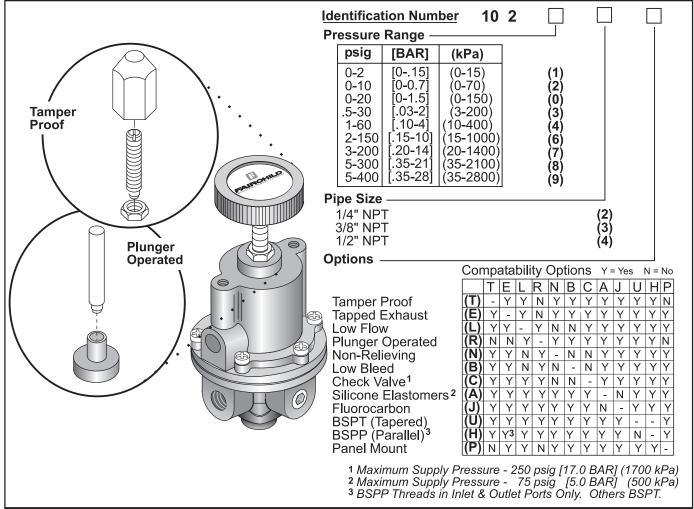
Figure 1. Model 10 Pneumatic Pressure Regulator Identification Number System.
