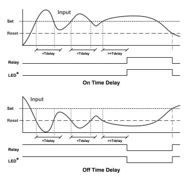
If the signal crosses the set point, the *On* time delay timer starts and the relay trips when the time delay has elapsed. If the signal drops below the set point (high alarm) before the time delay has elapsed, the *On* time delay timer resets and the relay does not change state. The same principle applies to the *Off* time delay.
