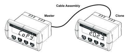
Figure 11. Meter Copy Connection
