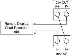
Figure 9. 4-20 mA Transmitter Powered by Meter
