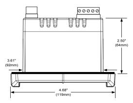
Figure 13. Case Dimensions - Top View
