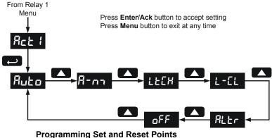
High alarm indication: program set point above reset point. Low alarm indication: program set point below reset point.
