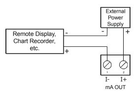
Figure 10. 4-20 mA Transmitter Powered Externally
