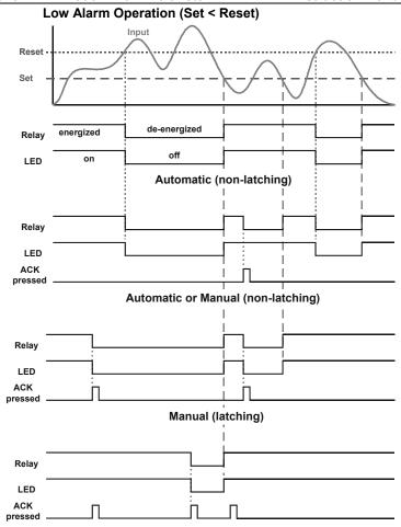
Manual only after passing above Reset (latching with clear)
