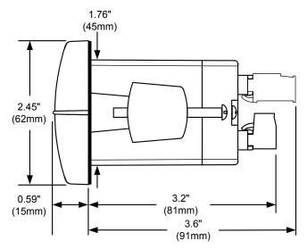
Figure 12. Meter Dimensions - Side View
