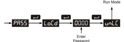
Entering the correct four-digit number sets the password to 0000, disabling the protection.
