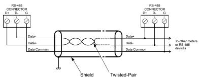
Figure 5. RS-485 Data Bus Connections
